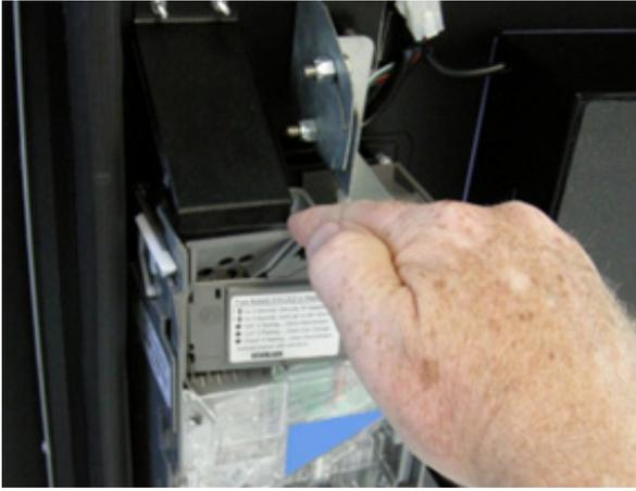
4. Check for coin jams in this area. Note: the ramp in this area should also be cleaned on a regular basis to ensure trouble-free operation.
