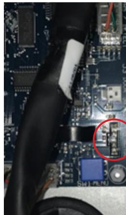
The Beverage Unit has a live product display that is lit by LED lighting. Locate the LED Light harness, **Figure 5**, on the inside of the Beverage Unit Door. Insert the LED Light harness up through the Snack Unit as done for the other connections. Connect the LED Light harness to the corresponding connector. Reinsert the Styrofoam piece for maximum insulation of the refrigeration unit.
